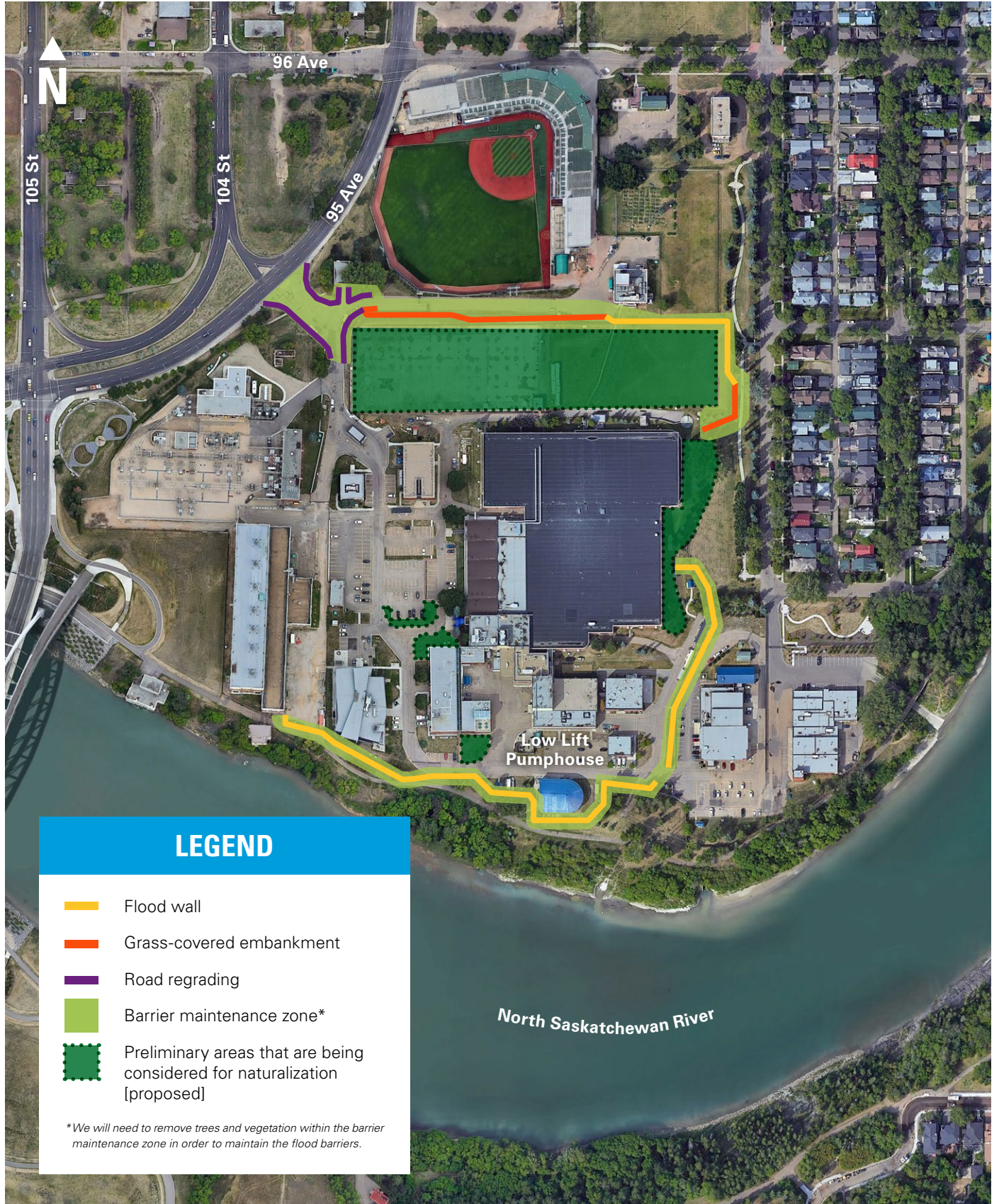
Figure 2. Infographic of Rosedale WTP plant site showing the expected impact from the flood mitigation project. We will plant pockets of vegetation around the plant site over time, such as at the areas marked for naturalization on the map.
