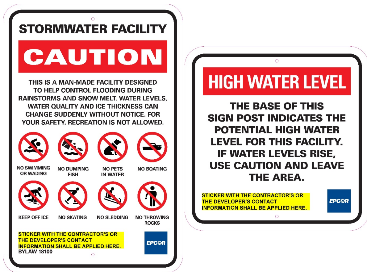
Figure 4.1: Wet SWMF Standard Safety Sign Example
