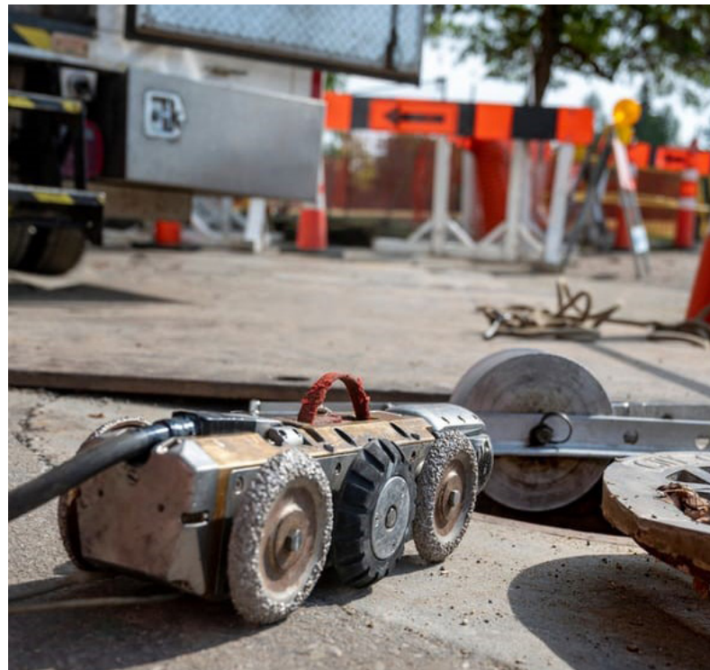
Televising equipment for inspecting wastewater pipes
