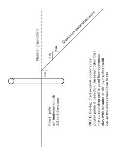
The area must be barricaded to avoid accidental contact with the digging equipment by other workers or the public. Employees must not stand or place anything directly on top of cables in the excavation when using excavation equipment (e.g. Hydrovac and Backhoe). At no time should anyone be closer than **1 m** to electrical equipment.
