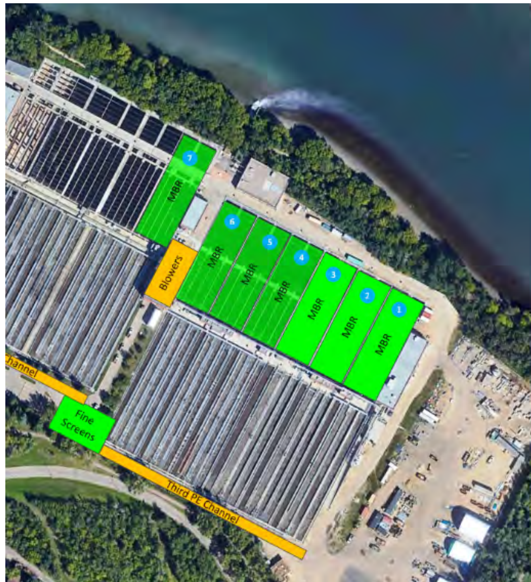
Starting in 2027 EPCOR will start retrofitting existing secondary clarifier tanks with membrane technology
