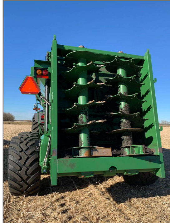
Photo 1: October 18, 2023. Agricultural spreader used to spread dewatered biosolids, cleaned prior to mobilization to Sturgeon County fields.
